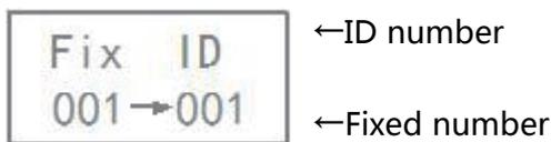
In this interface press left / right key can modify the number status , press plus/minus key or number key can modify numbers , The front of number refers to the initial controller' s number , the next number refers to the end of the controller , after modify ok press
