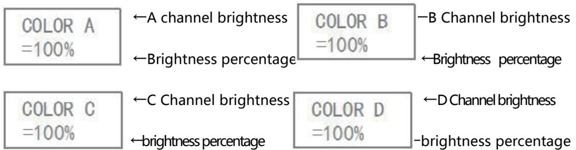
In this interface press plus / minus setting each channel brightness , press again
