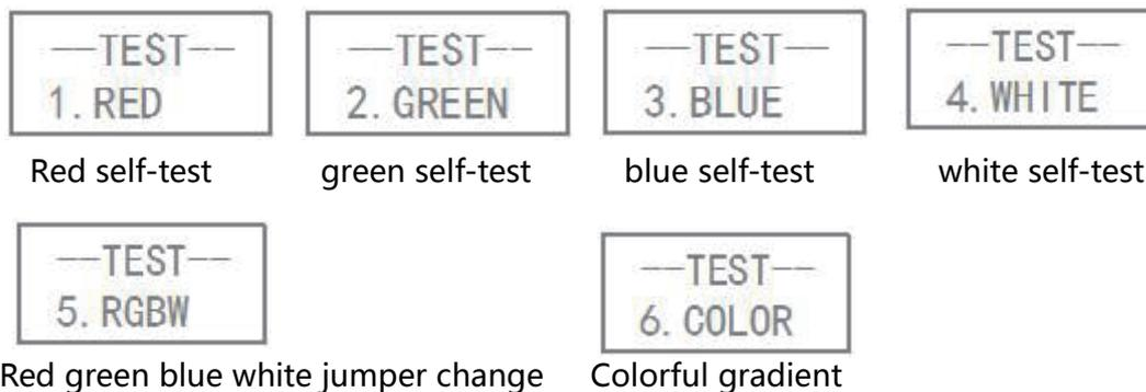
Note: In the process of self-test process ,press
