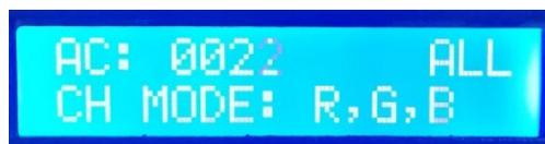
2.8. Press the “**MODE**” button again to enter the “**MC**” manual test mode. “**SPEED+**” and “**SPEED-**” can adjust the pixel points (long press “speed+” or “speed-” can be quickly incremented or
