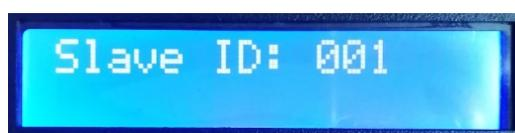
2.3. After completing the number setting, press the "SET/Save" button to start the numbering.
