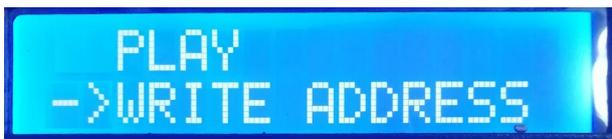
2.3. Press “**SET**” button to select “**WRITE ADDRESS**”, enter into address writing mode interface, as show in the figure:
