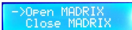
3.1.4. Press the “**SPEED+**” and “**SPEED-**” buttons to move the arrow up and down to select the On/Off option.
