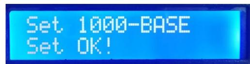
5.6. Select to complete the transmission rate selection, press “**SET**” to exit and return to the main interface.
