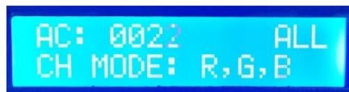
3.5. Press **"MODE"** to switch the testing channel slection;
