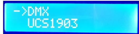
3.3.4. Press the “**SPEED+**” and “**SPEED-**” buttons to move the arrow up and down to select the IC option.
