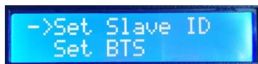
2.2. Press the "SET" button again, the main control display enters the numbering page, the "SPEED+" button and the "SPEED-" button adjust the number of the starting sub-control, as shown below:
