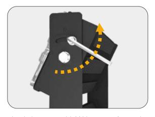
Lock the screw with M6 hexagonal wrench
