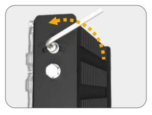
Loosen the screw with M6 hexagonal wrench
