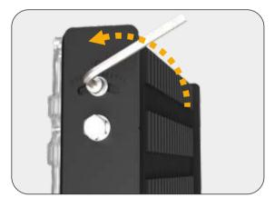
Loosen the screw with M6 hexagonal wrench
