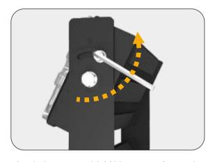
Lock the screw with M6 hexagonal wrench
