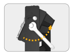
Lock the screw with M8 wrench
